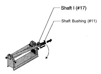
Figure 4 -- Removing Partial Rolls
